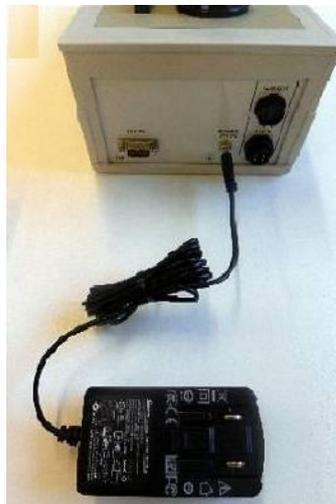
Fig. 8 Power cord connection of peristaltic pump
