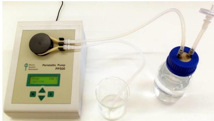
Fig. 7 Basic configuration of Peristaltic Pump
