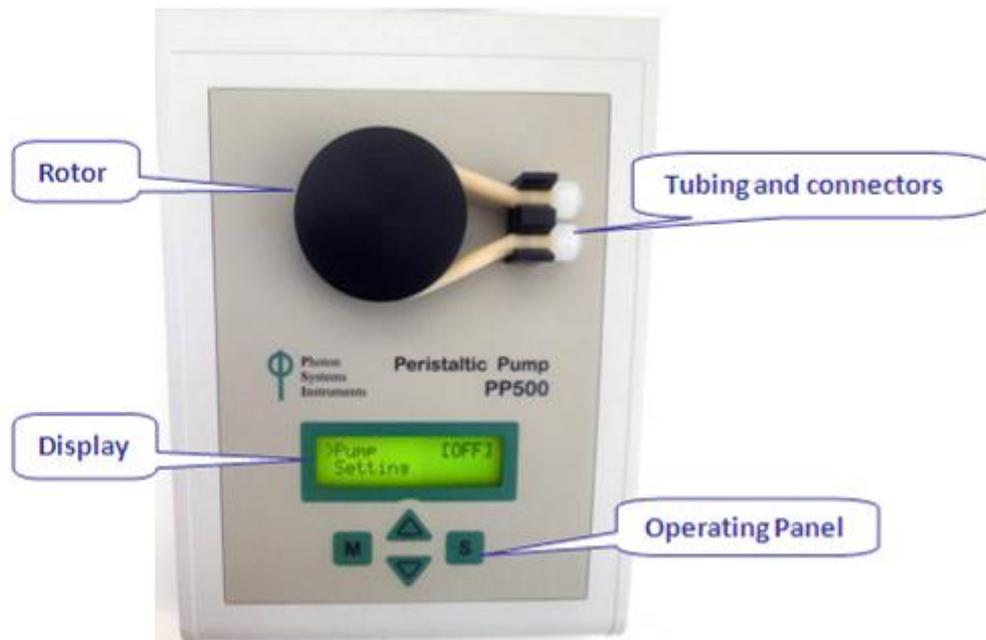
Fig. 4 Front panel
