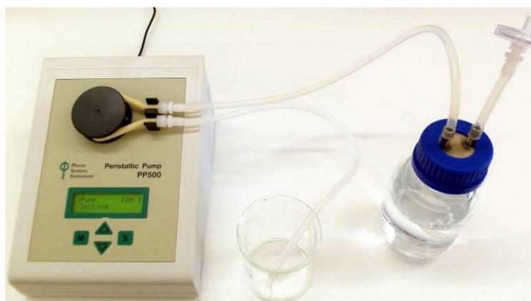
Fig. 11 Basic configuration of Peristaltic Pump for flow rate calibration
