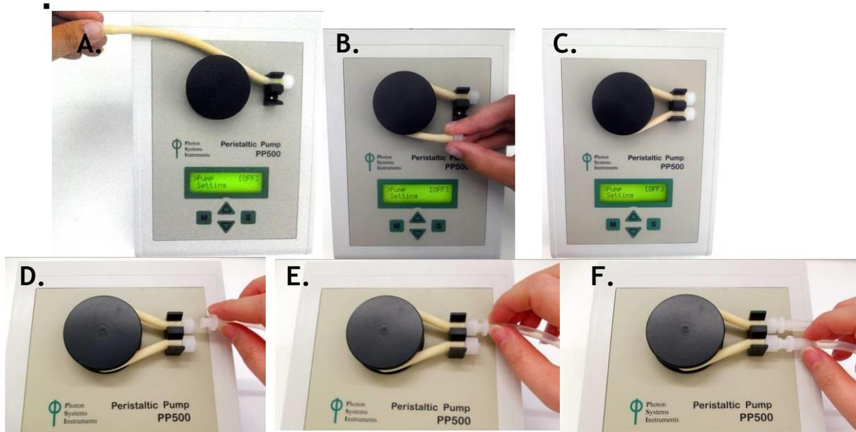
Fig. 6 Assembly of the peristaltic pump
