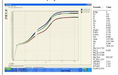
Measured data are sequentially stored in the FluorPen memory and may be recalled for transcription to a computer.
